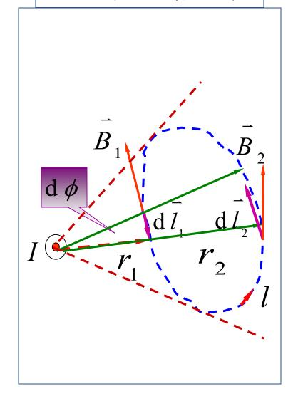
$$B_1 = \frac{\mu_0 I}{2\pi r_1}, \quad B_2 = \frac{\mu_0 I}{2\pi r_2}$$
